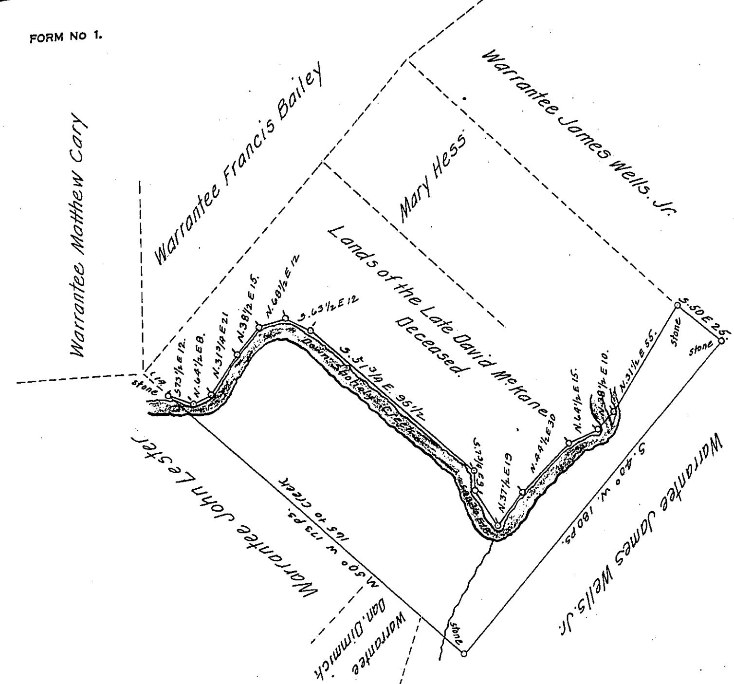
A Draft of a tract of land situated in the Township of Shohola and County of Pike, containing Seventy three acres, fifty four perches and allowance of six percent for roads, etc. Surveyed for Henry W. Richardson the 6<sup>th</sup> day of June 1908. it being part of a larger tract containing One hundred ninetynine acres.
